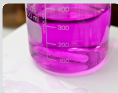
Glass-ceramic plate with high chemical resistance. It is also suitable for observing color changes (e.g. during titration, etc.).
